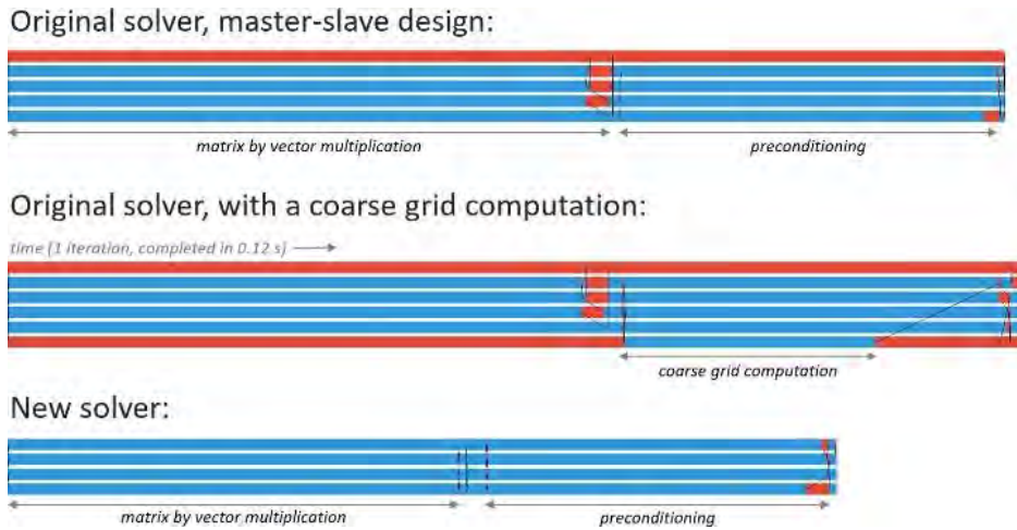
Fig. 1. Traces of one PCG iteration processing four subdomains. From top, records for the original solver with AS1 and AS2, and new solver with AS1 only. States of parallel processes: work (blue), wait or idle (red)
