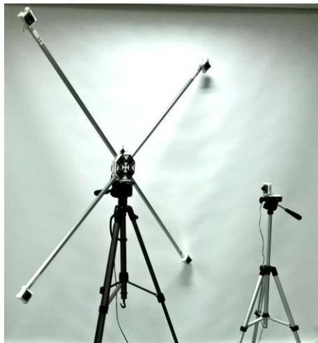
Fig. 1. Hexamite ultrasonic positioning system architecture
