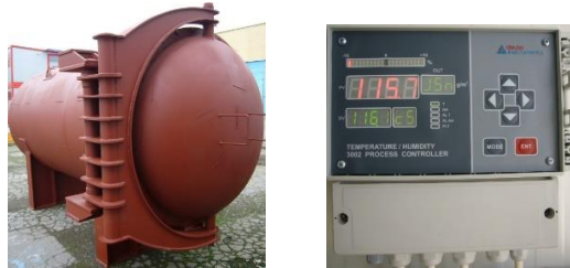
Fig. 16. Autoclave (left) and PLC in a system for model-based control of the wood steaming process in it (right)
