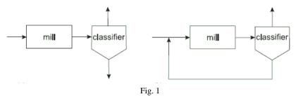
In the first case the output material is simply separated in fractions with different particle sizes and the grinding process is actually not affected by the classifier. In the second case the classifier returns coarse material back to the mill feed and only the fine product is obtained at the output of the grinding circuit. In practice various types of interconnections between mills and classifiers are possible aimed at increasing the grinding efficiency of the overall process.
