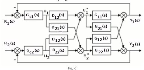
The system is described by the vector-matrix equations  $U = G_C(R - Y)$ ,  $U^* = DU$ ,  $Y = GU^*$  which give the input-output equation
