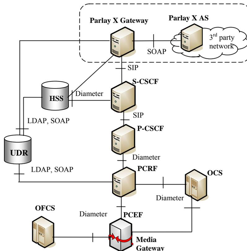
Fig. 1. Deployment of Parlay X Web Services in PCC architecture
