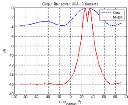
Fig. 6. Signal azimuth separation by the UCA
