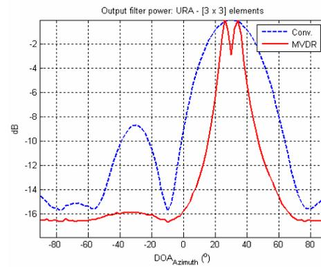
Fig. 5. Signal azimuth separation by the URA
