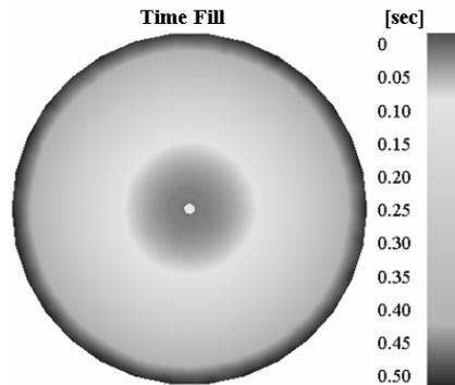
Fig. 6. Mould filling pattern (modified sprue system):  $T_{\text{melt}} = 320 \text{ }^{\circ}\text{C}$ ;
