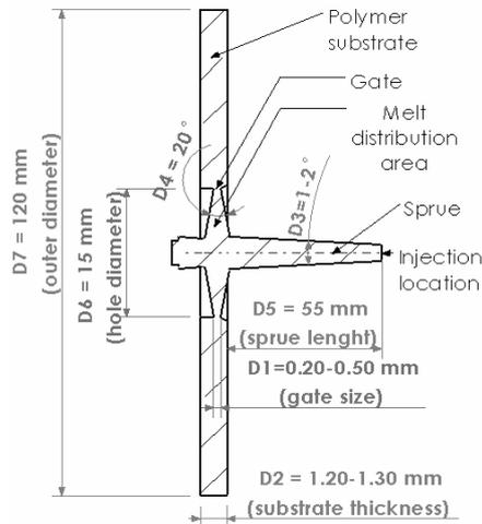
Fig. 5. Cross-section of the polymer substrate and a modified sprue system
