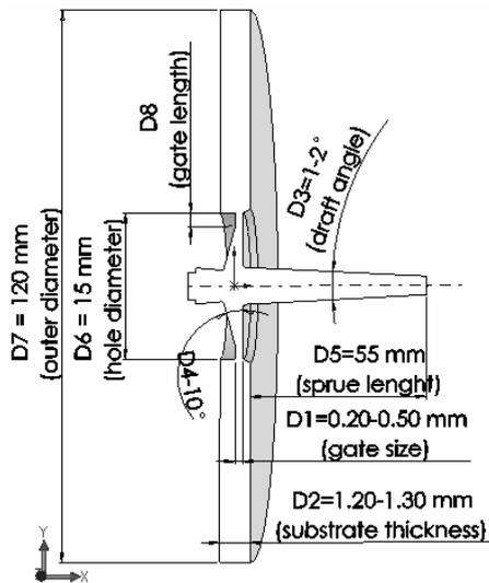
Fig. 3. Integrated 3D CAD model of the polymer substrate and a conventional sprue system
