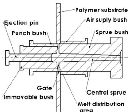
Fig. 2. Cross-section of the conventional sprue system design
