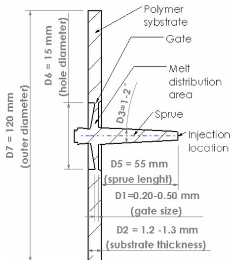
Fig. 4. Cross-section of the polymer substrate and a conventional sprue system with gate length  $D6 = 0.00$  mm
