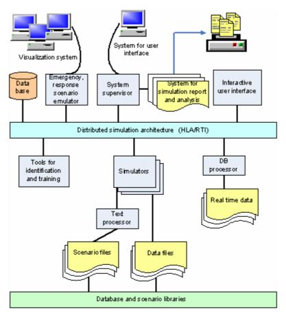
Fig. 5. Simulation architecture for CAX
