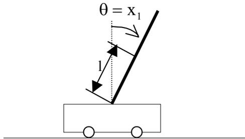
Fig. 1. The inverted pendulum system
