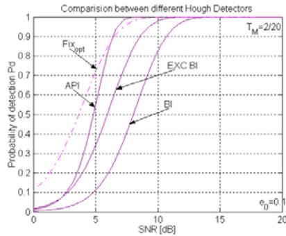
Fig. 15. Probability of detection for Hough detectors with two-dimensional CFAR processors, at a value  $e_0 = 0.1$
