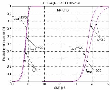
Fig. 8. Probability of detection of a Hough detector with EXC CFAR BI processor, for  $T_M=7/20$  and  $T_M=13/20$
