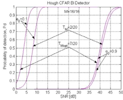
Fig. 3. Average detection threshold of the Hough detector compared to the optimal detection threshold in the Hough parameter space
