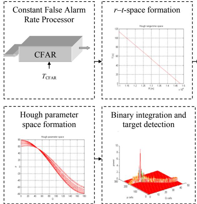
Fig. 1. The general structure of an adaptive Hough detector
