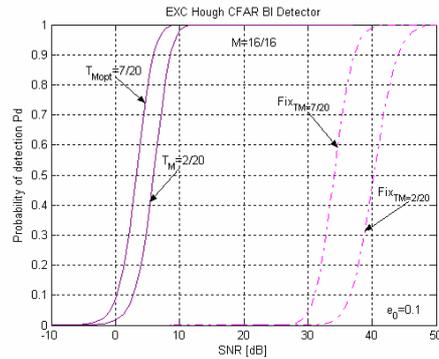
Fig. 9. Probability of detection of a Hough detector with EXC CFAR BI processor, for  $T_M=2/20$ ,  $T_M=7/20$  and  $e_0=0.1$
