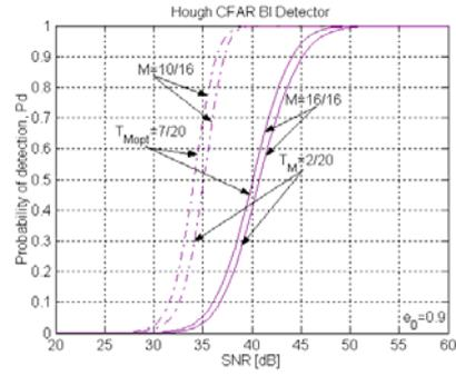
Fig. 4. Profits of the Hough detector (dashed line), for value of  $T_M=2$  and for an optimal value  $T_M=7$ , for  $e_0=0.9$ , compared to the Hough detector (solid line) for another binary rule
