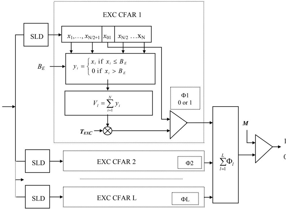
Fig. 7. Block diagram of an EXC CFAR processor with binary integration
