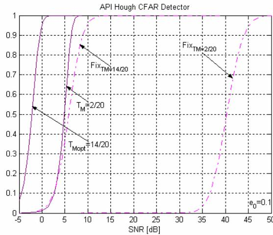
Fig. 12. Probability of detection of a Hough detector with API CFAR processor for  $T_M=2/20$ ,  $T_M=14/20$  and  $e_0=0.1$
