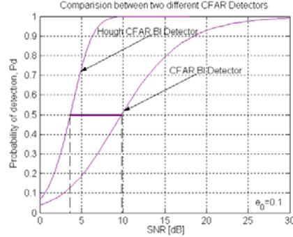
Fig. 6. Profits of using the Hough detector with CFAR BI processor, compared to using the CFAR BI processor
