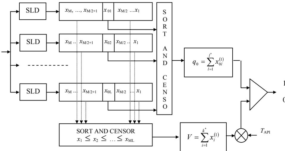
Fig. 11. Block diagram of active API CFAR processor
