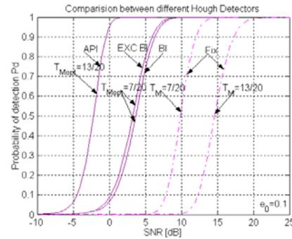
Fig. 16. Probability of detection for Hough detector with two-dimensional CFAR processors, at different values of  $T_{Mopt}/N_s$
