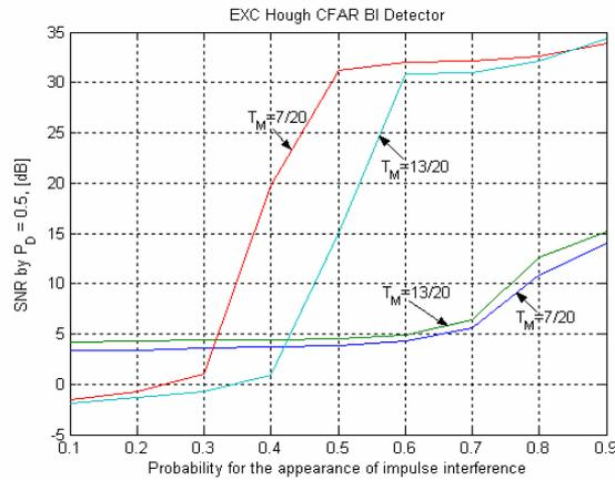
Fig. 10. ADT of an EXC Hough CFAR BI detector for optimal values of detection threshold  $T_M=7$  and  $T_M=13$  for binary rules  $M$ -out-of- $L = 16/16$  (solid line) and  $M$ -out-of- $L = 10/16$  (dashed line)
