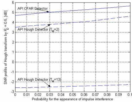
Fig. 14. Profits of the API Hough detector (dashed line), for optimal value of detection threshold  $T_M=13$  and for value  $T_M=2$ , compared to the API CFAR detector (solid line) for  $L=16$
