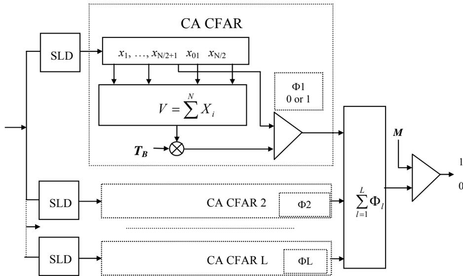
Fig. 2. Block-diagram of a CFAR processor with binary integration
