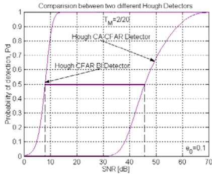
Fig. 5. Profits of using the Hough detector with CFAR BI processor, compared to using the Hough detector with CA CFAR processor
