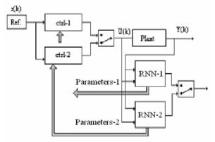
Fig. 2. Block-diagram of the indirect adaptive fuzzy-neural multi-model control system
