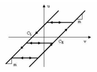
Fig. 3. Backlash model, where: v(t) is the input and u(t) is the output;  $C_{R} > 0$  is the right path and  $C_{L} < 0$  is the left path
