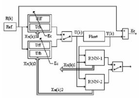
Fig. 1. Block-diagram of a direct adaptive fuzzy-neural multi-model control system
