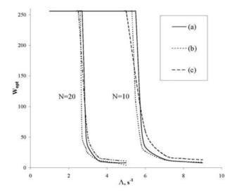
Fig. 9. Backoff window optimal for:  $a - M_u$ ;  $b - T^{MAC}_{\ u}$  and  $c - T^{MAC}_{\ u} + T^{MAC}_{\ d}$  versus traffic rate with q = 0.1
