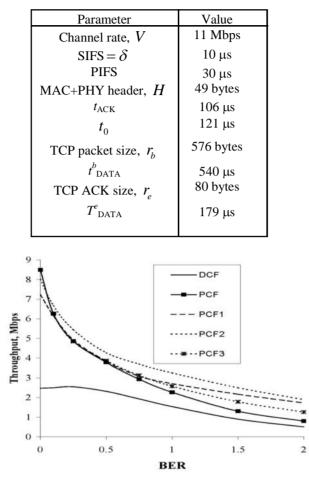
Fig. 5. Comparison of DCF and PCF with packet integration
