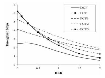
Fig. 4. Comparison of DCF and PCF for BER  $\times 10^4$  and N = 3
