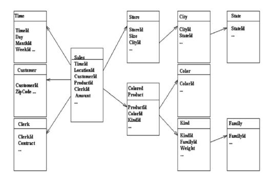
Fig. 4. An example of a snowflake schema [2]
