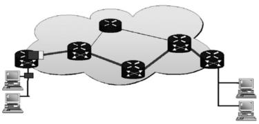
Fig.1. IP Network with LERs and an IP packet with header attached
