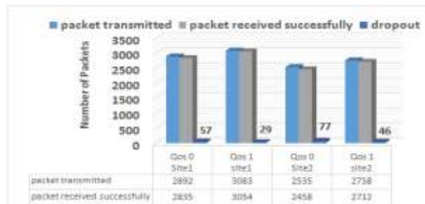
Fig. 10. System performance over an MQTT protocol: rooftop (Site 1 – outdoor) and home (Site 2 – indoor)
